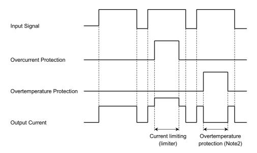
Note2: The overheating detector circuits feature hysteresis. After overheating is detected, normal operation is restored only when the channel temperature falls by the hysteresis amount (5°C typ.) in relation to the overheating detection temperature.
