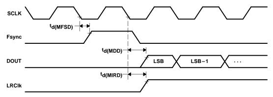
Figure 4-4. SCLK to Fsync, DOUT, and LRClk - Master Mode 7
