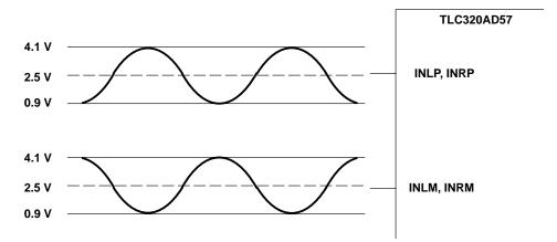
Figure 2–2. Differential Analog Input Configuration
