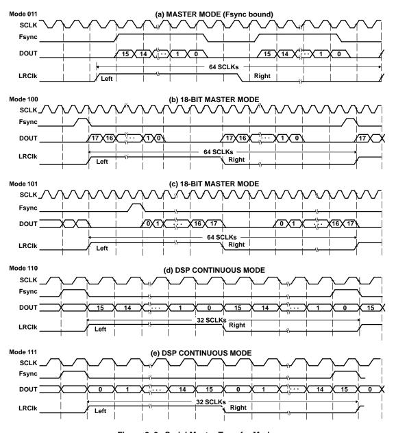
Figure 2-3. Serial Master Transfer Modes
