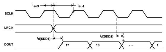
Figure 4–5. SCLK to LRCIk and DOUT – Slave Mode 0, Fsync High
