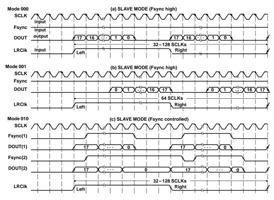
Figure 2-4. Serial Slave Transfer Modes
