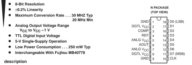
The TL5602 is a low-power ultra-high-speed video digital-to-analog converter that uses the Advanced Low-Power Schottky (ALS) process. It converts digital signals to analog signals at a sampling rate of dc to 20 MHz. Because of such high-speed capability, the TL5602 is suitable for digital video applications such as digital television, video processing with a computer, and radar signal processing.
