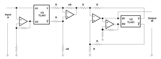
NOTE: R designates resistors of equal value, typically 2 k $\Omega$  to 10 k $\Omega$ . The power to which the input variable is raised is fixed by setting nR. Output W may need to be amplified to give the correct value.
