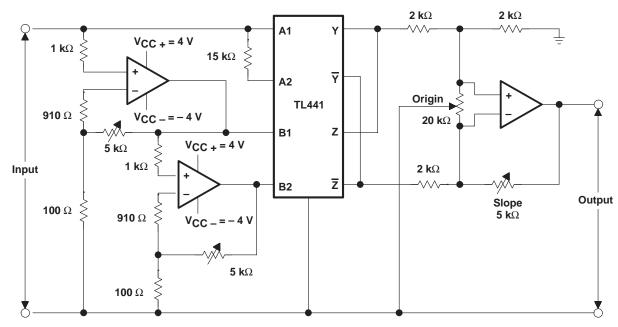
NOTES: A. Inputs are limited by reducing the supply voltages for the input amplifiers to  $\pm 4$  V.
