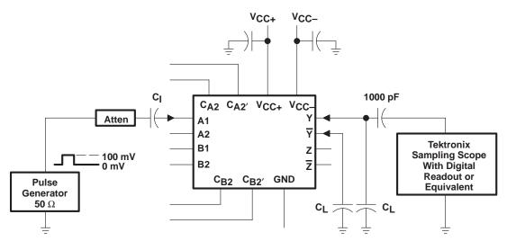
NOTES: A. The input pulse has the following characteristics:  $t_W = 200 \text{ ns}, t_f \le 2 \text{ ns}, t_f \le 2 \text{ ns}, PRR \le 10 \text{ MHz}.$
