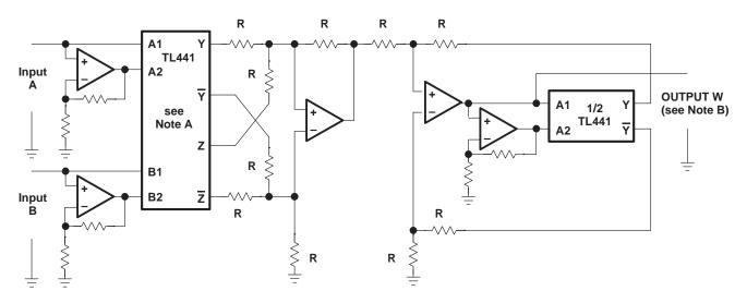
NOTES: A. Connections shown are for multiplication. For division, Z and  $\overline{Z}$  connections are reversed.
