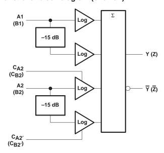
$\begin{array}{l} Y \propto log~A1 + log~A2;~Z \propto log~B1 + log~B2\\ where:~A1,~A2,~B1,~and~B2~are~in~dBV,~0~dBV = 1~V.\\ C_{A2},~C_{A2'},~C_{B2},~and~C_{B2'}~are~detector~compensation~inputs. \end{array}$
