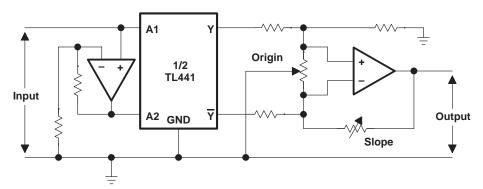
Figure 12. Output Slope and Origin Adjustment
