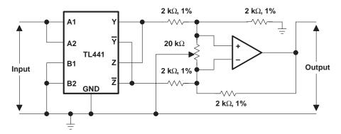
Figure 14. Utilization of Paralleled Inputs
