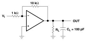
Figure 2. Gain-of-10 Inverting Amplifier
