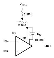
Figure 4. Input Offset Voltage Null Circuit
