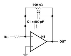
Figure 3. Feed-Forward Compensation
