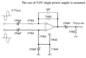
Figure 13: Differential input signal application
