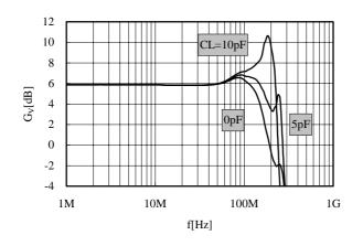
Figure 10: Frequency characteristics of capacitive load
