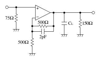
Figure 9: Measurement circuit
