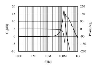
Figure 12: Frequency characteristic of buffer amplifier
