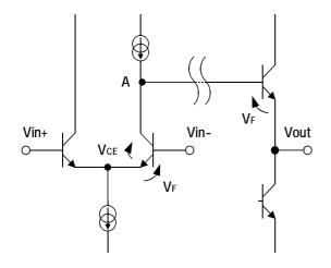
Figure 1: The internal equivalent circuit
