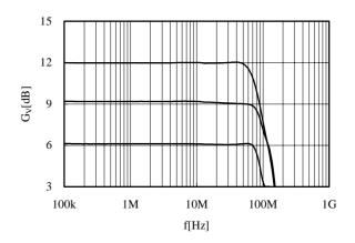
Figure 8: 30MHz flatness characteristics
