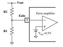
Fig1: Setting the output voltage
