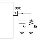
Fig 4. Oscillator pin connection
