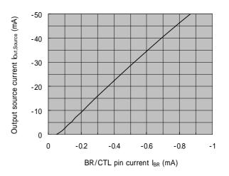
Fig 8. Output source current vs. BR/CTL pin current
