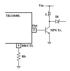
Fig6: Programming output current
