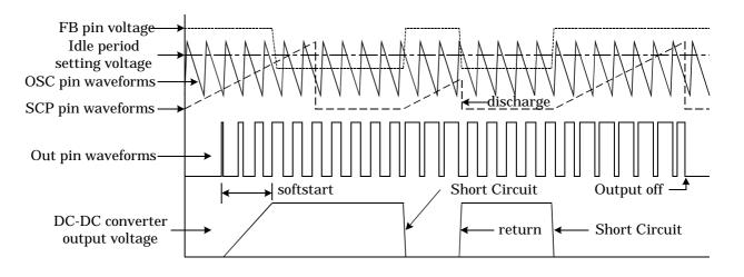
Fig.11: Timing Diagram of soft start and short circuit detection.
