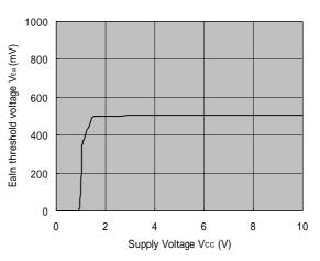
EaIn threshold voltage variation ratio vs. Supply voltage  $T_a=25^{\circ}C$
