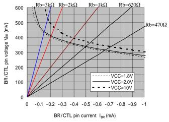
Fig 7. BR/CTL pin voltage vs. BR/CTL pin current
