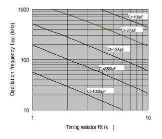
Fig.3: Oscillator frequency vs. Timing resistor
