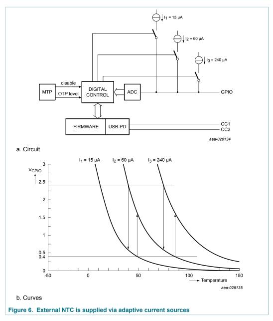
The voltage on the GPIO pin is measured via an internal A-to-D converter. If the voltage on the GPIO pin drops to below 400 mV, the source current is increased. If the voltage on the GPIO pin exceeds 2.4 V, the source current is decreased. When a 47 k $\Omega$  NTC resistor with a Beta of 4108 is used, the temperature is accurately measured with a better than < 5 °C accuracy within a range of 0 °C to > 120 °C.
