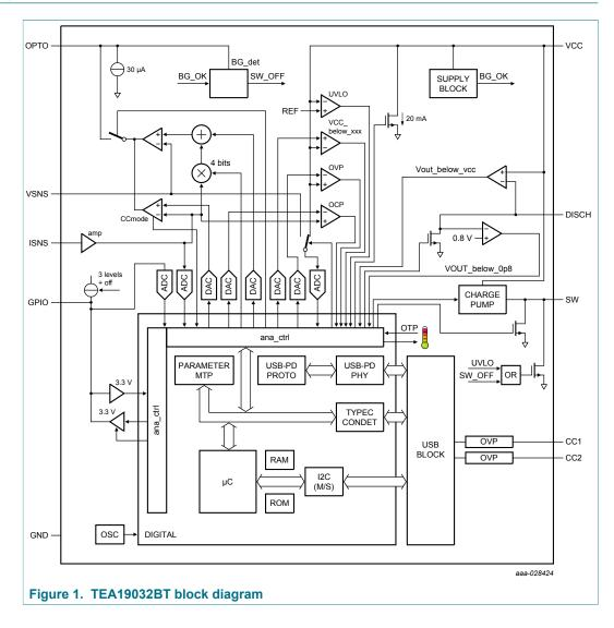
USB-PD 2.0/USB-PD 3.0/QC 4 controller for SMPS
