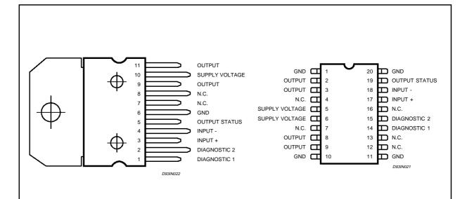
Note: Output pins must be must be connected externally to the package to use all leads for the output current (Pin 9 and 11 for Multiwatt package, Pin 2, 3, 8 and 9 for PowerSO20 package).
