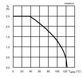
Figure 8: Max. Output Current vs. Ambient Temperature (Multiwatt with heatsink,  $R_{th j-amb} = 15$ °C/W)
