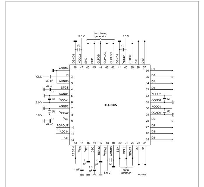
Depending on the application, the following connections must be made:
