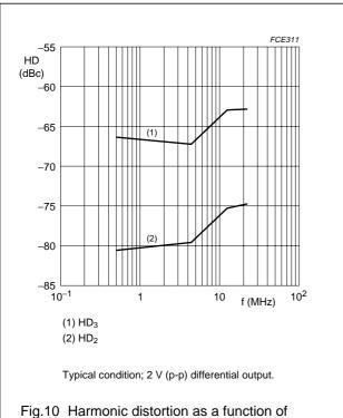
Fig.10 Harmonic distortion as a function of frequency for minimum gain plus 24 dB.
