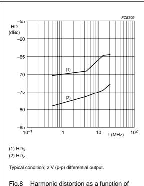
Fig.8 Harmonic distortion as a function of frequency for minimum gain plus 12 dB.
