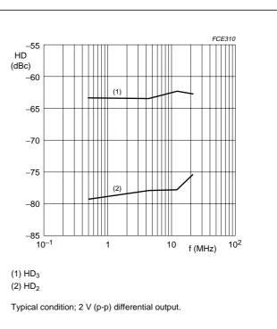
Fig.9 Harmonic distortion as a function of frequency for minimum gain plus 18 dB.
