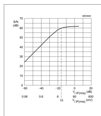
Fig.5 Typical signal-to-noise ratio as a function of IF input voltage.
