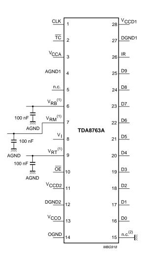
The analog and digital supplies should be separated and decoupled.
