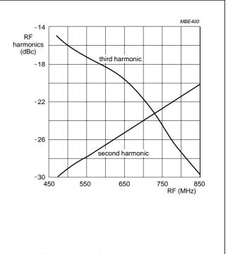
Fig.12 Typical level of RF harmonics for an asymmetrical application.
