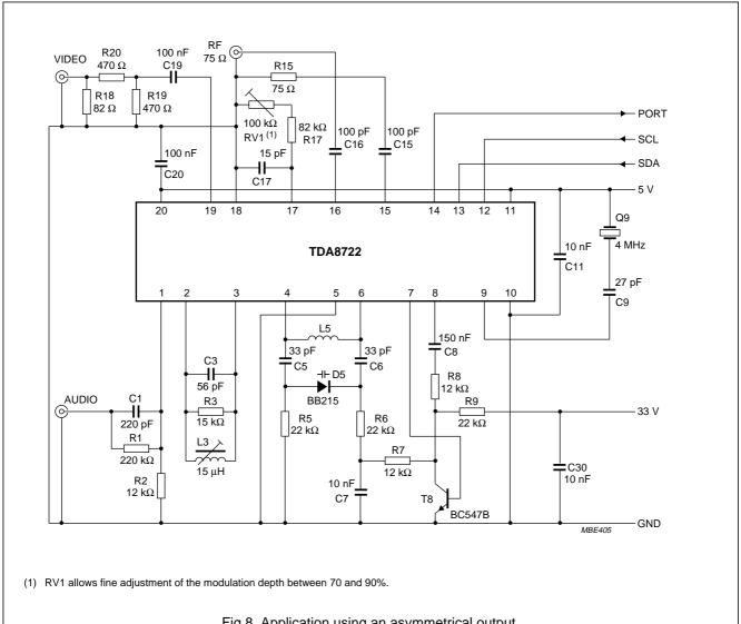
Fig.8 Application using an asymmetrical output.
