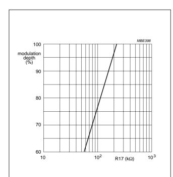
Fig.10 Typical modulation depth as a function of the value of R17.
