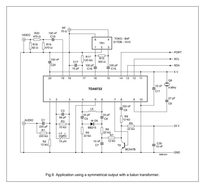
In the design of the application, it is highly recommended to separate the part of the RF oscillator as much as possible from the part of the RF outputs in order to avoid parasitic coupling between these two parts.
