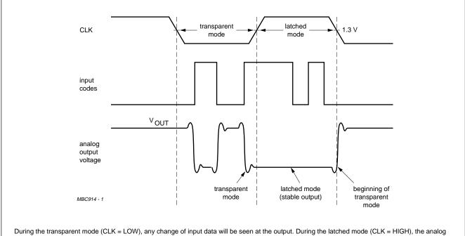
During the transparent mode (CLK = LOW), any change of input data will be seen at the output. During the latched mode (CLK = HIGH), the analog output remains stable regardless of any change at the input. A change of input data during the latched mode will be seen on the falling edge of the clock (beginning of the transparent mode).
