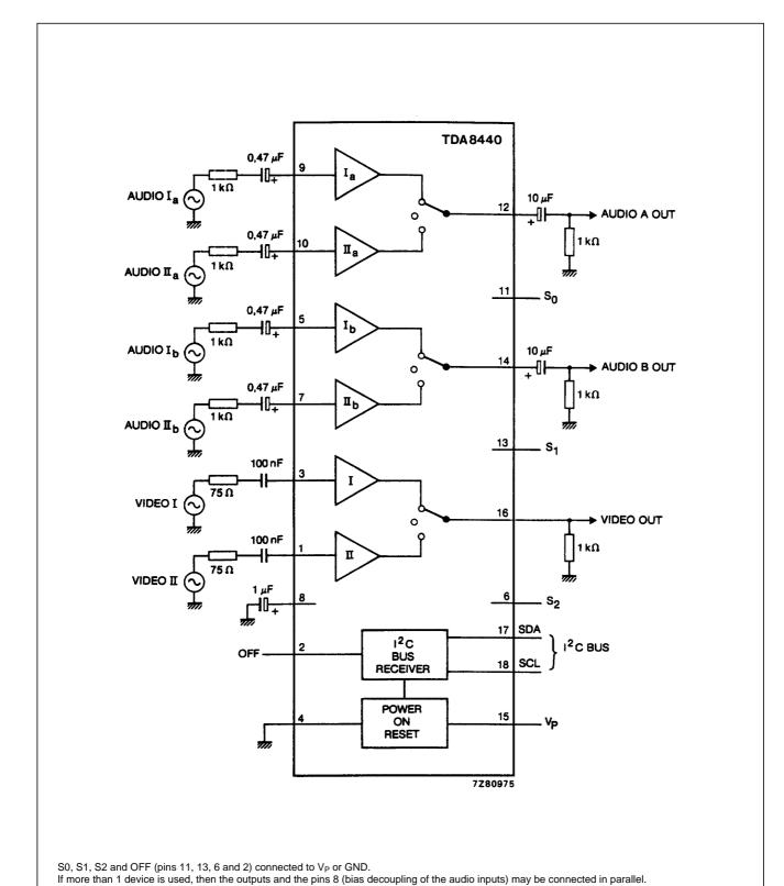
Fig.1 Block diagram and test circuit.
