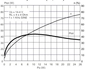
Figure 13. Power Dissipation vs. Average Ouput Power (Audio Program Simulation, 2Ω)
