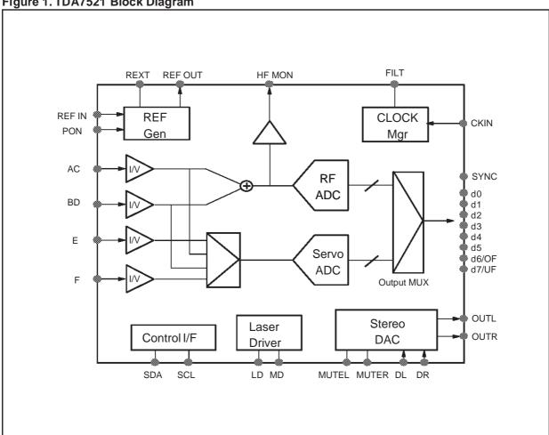
Figure 1. TDA7521 Block Diagram
