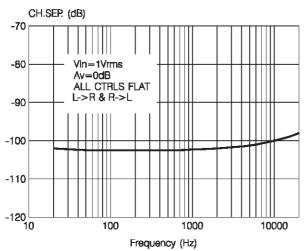
Figure 4: Channel separation vs. frequency
