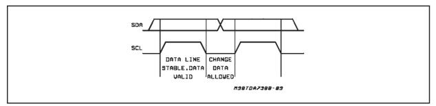
Figure 4: Timing Diagram of I<sup>2</sup>CBUS
