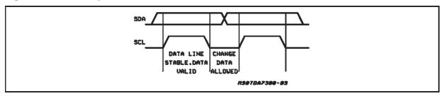
Figure 4. Timing Diagram of I<sup>2</sup>CBUS
