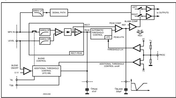
Figure 3: Block Diagram of the Noise Blanker
