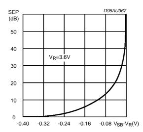
frequency is reduced down to 1kHz to improve the signal to noise ratio. Furthermore the conditions of the stereo separation (see fig.2) can be controlled through the signal applied to Pin 16 (VSB). Both signal levels (VSB and VHCC) are referred to Pin 17 (VR), with the characteristic that the control range is 11% of VR.
