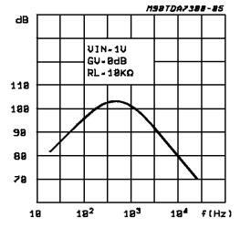
SGS-THOMSON MICROELECTRONICS Figure 9: Input Separation (L1 - L2) vs. Frequency
