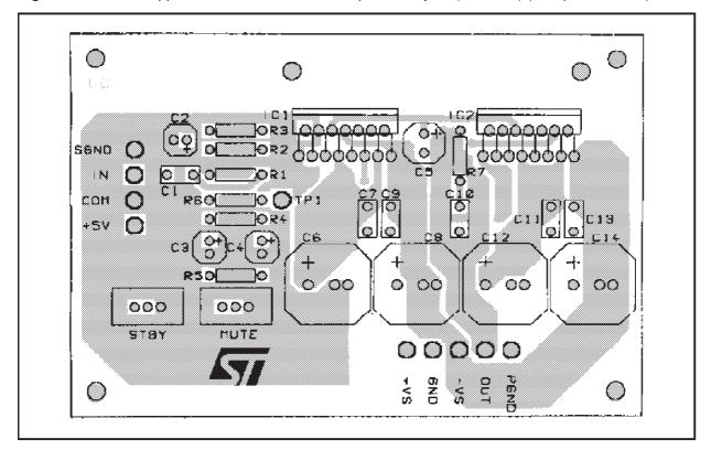
Figure 7a: Modular Application P.C. Board and Component Layout (scale 1:1) (Component SIDE)
