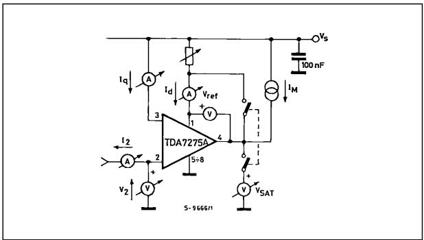
Figure 2: Application Circuit.
