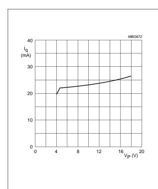
Fig.3 Quiescent current as a function of supply voltage.
