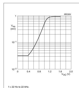
Fig.9 Noise voltage as a function of volume control voltage.
