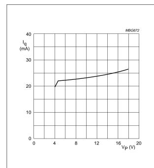
Fig.3 Quiescent current as a function of supply voltage.
