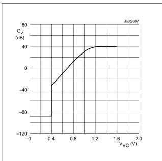
Fig.8 Voltage gain as a function of volume control voltage.
