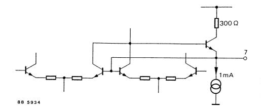
Pin 7 AF-output AM/FM (channel 1, 5.5 MHz)
