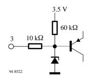
Figure 6. Input selector switch (Pin 3)
