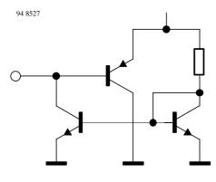
Figure 11. Tuner AGC – output (Pin 11)
