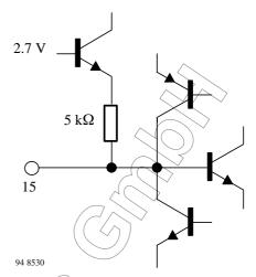
Figure 14. Black level capacitor (Pin 15)
