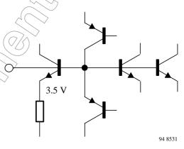
Figure 15. Internal reference voltage (Pin 17)
