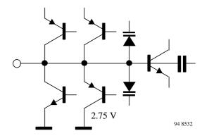
Figure 16. Loop filter (Pin 18)
