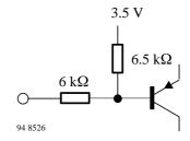
Figure 10. Tuner AGC – take over point (Pin 10)
