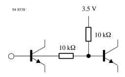
Figure 22. VCO offset compensation (pin 26)
