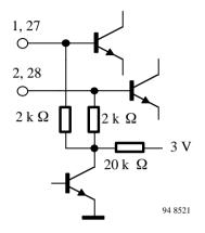
Figure 5. Sound IF inputs (pin 1-2, 27-28)
