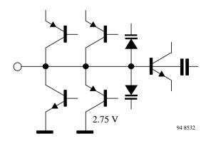
Figure 16. Loop filter (pin 18)
