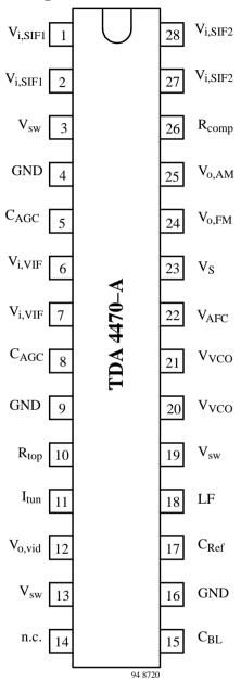
Figure 2. Pin configuration
