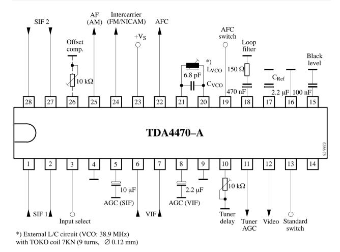
Figure 3. Test circuit
