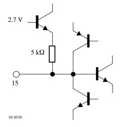
Figure 14. Black level capacitor (pin 15)
