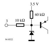
Figure 6. Input selector switch (pin 3)
