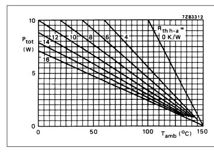
$\label{eq:fig:constraints} \begin{array}{ll} Fig.2 & Total power dissipation. \\ R_{th \; h\text{-}a} \; \text{includes} \; R_{th \; mb\text{-}h} \\ & \text{which is expected when heatsink compound is used.} \\ R_{th \; j\text{-}mb} \leq 5 \; \text{K/W}. \end{array}$
