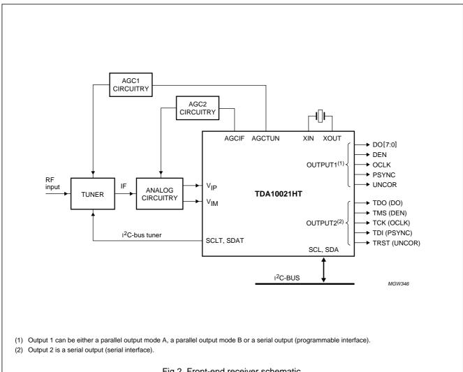
Fig.2 Front-end receiver schematic.
