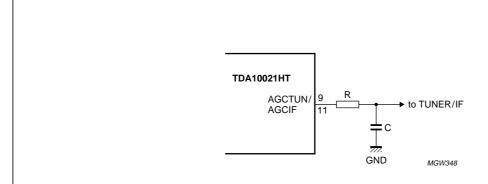
R and C are chosen to verify  $\frac{SR}{1024} < f_c < \frac{XIN}{16}$  with R = 1.5 k $\Omega$  and C = 1 nF,  $f_c$  = 100 kHz.
