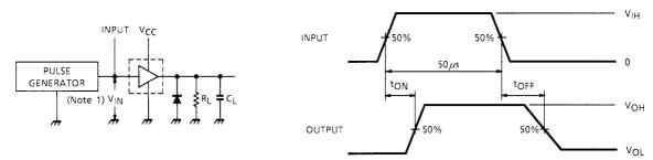
Note 1: Pulse width 50  $\mu$ s, duty cycle 10% Output impedance 50  $\Omega$ , t<sub>r</sub> ≤ 5 ns, t<sub>f</sub> ≤ 10 ns Note 2: C<sub>L</sub> includes probe and jig capacitance
