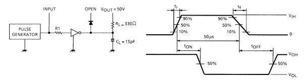
Note 1: Pulse Width 50  $\mu$ s, Duty Cycle 10% Output Impedance 50  $\Omega$ , t<sub>r</sub> ≤ 5 ns, t<sub>f</sub> ≤ 10 ns Note 2: See below
