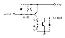
Note: The input and output parasitic diodes cannot be used as clamp diodes.
