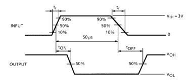
Note 1: Pulse Width 50  $\mu$ s, Duty Cycle 10% Output Impedance 50  $\Omega$ , tr  $\leq$  5 ns, tf
