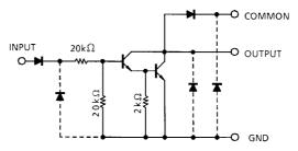
Note: The input and output parasitic diodes cannot be used as clamp diodes.
