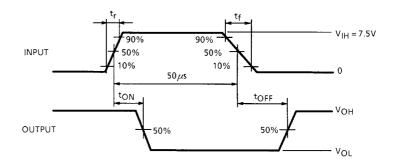
Note 1: Pulse Width 50  $\mu$ s, Duty Cycle 10% Output Impedance 50  $\Omega$ , t<sub>f</sub> ≤ 5 ns, t<sub>f</sub> ≤ 10 ns Note 2: C<sub>L</sub> includes probe and jig capacitance.
