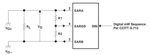
Figure 6. Gain-Setting Configuration
