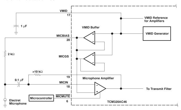
Figure 1. Typical Microphone Interface
