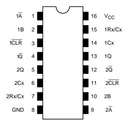
Note: When using a single circuit only, please set  $\overline{CLR}$  to L, keep  $Rx/Cx \cdot Q \cdot \overline{Q}$  open and set other pins to either H or L.
