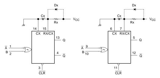
Note1: Cx, Rx, Dx are external capacitor, resistor, and diode, respectively.
