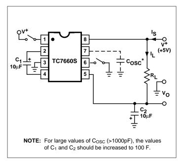
Figure 1. TC7660S Test Circuit
