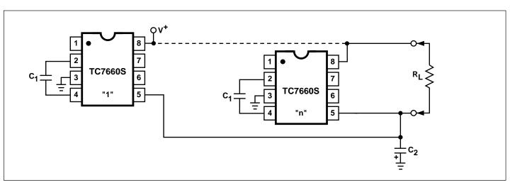
Figure 4. Paralleling Devices Lowers Output Impedance
