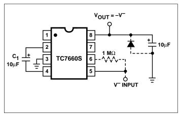
Figure 10. Positive Voltage Multiplier
