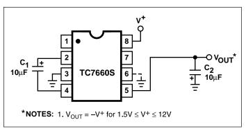
Figure 3. Simple Negative Converter
