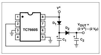
Figure 8. Positive Voltage Multiplier
