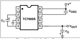
Figure 7. Lowering Oscillator Frequency
