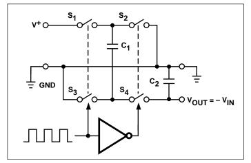
Figure 2. Idealized Charge Pump Inverter
