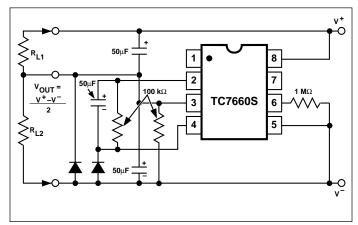
Figure 11. Splitting a Supply in Half
