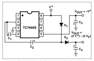
Figure 9. Combined Negative Converter and Positive Multiplier
