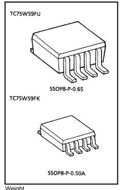
Weight SSOP8-P-0.65: 0.021g (typ.) SSOP8-P-0.50A: 0.01g (typ.)
