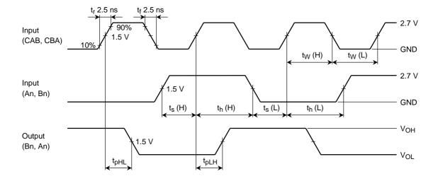
Figure 5  $t_{pLH}$ ,  $t_{pHL}$ ,  $t_w$ ,  $t_s$ ,  $t_h$
