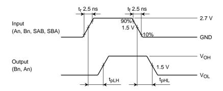
Figure 2 t<sub>pLH</sub>, t<sub>pHL</sub>
