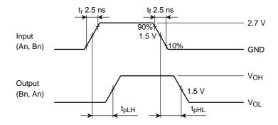
Figure 2 t<sub>pLH</sub>, t<sub>pHL</sub>
