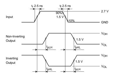
Figure 2 t<sub>pLH</sub>, t<sub>pHL</sub>
