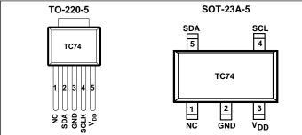
Communication with the TC74 is accomplished via a simple 2-wire SMBus/I<sup>2</sup>C-compatible serial port. This bus also can be used to implement multi-drop/multi-zone monitoring. The SHDN bit in the CONFIG register can be used to activate the low-power Standby mode.
