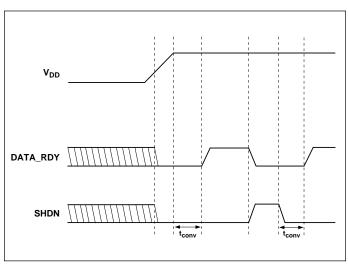
Figure 2. DATA\_RDY, SHDN Operation Logic Diagram
