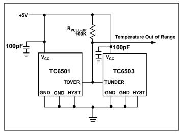
Figure 1. Over and Under Temperature Alarm
