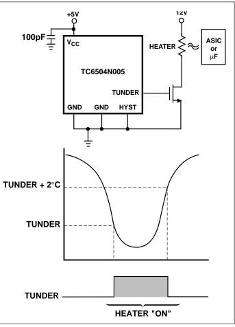
Figure 3. TC6504N005 As Heater Thermostat
