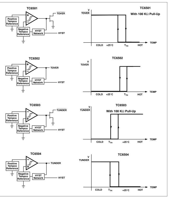
Figure 4. Functional Block Diagrams
