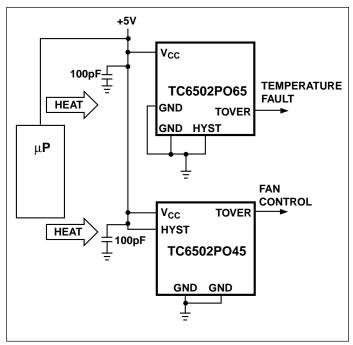
Figure 2. Fan Control Circuit with Over Temperature Alert
