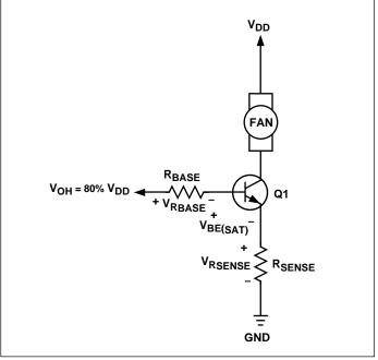
Figure 5. Circuit for Determining  $R_{\mbox{\scriptsize BASE}}$
