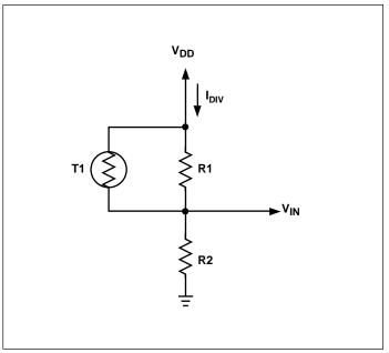
IDIV Figure 4. V<sub>AS</sub> Circuit Figure 3. Temperature Sensing Circuit
