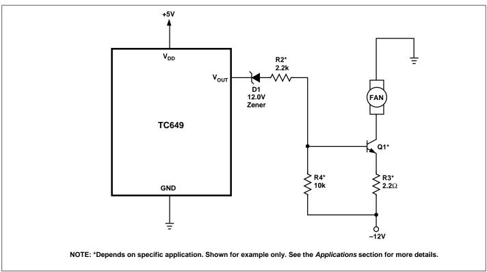
Figure 9. Powering the Fan from a Negative Supply
