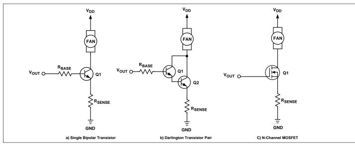
Figure 8. Output Drive Transistor Circuit Topologies
