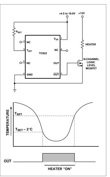
Figure 5. TC622 as a Heater Thermostat
