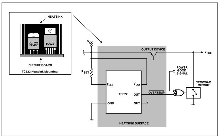
Figure 3. TC622 Power Supply Over-Temperature Shutdown
