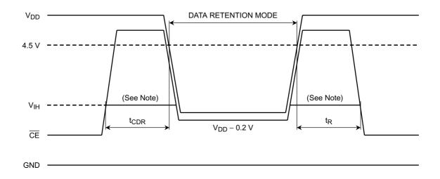
Note: When  $\overline{\text{CE}}$  is operating at the V<sub>IH</sub> level (2.2V), the standby current is given by I<sub>DDS1</sub> during the transition of V<sub>DD</sub> from 4.5 to 2.4V.
