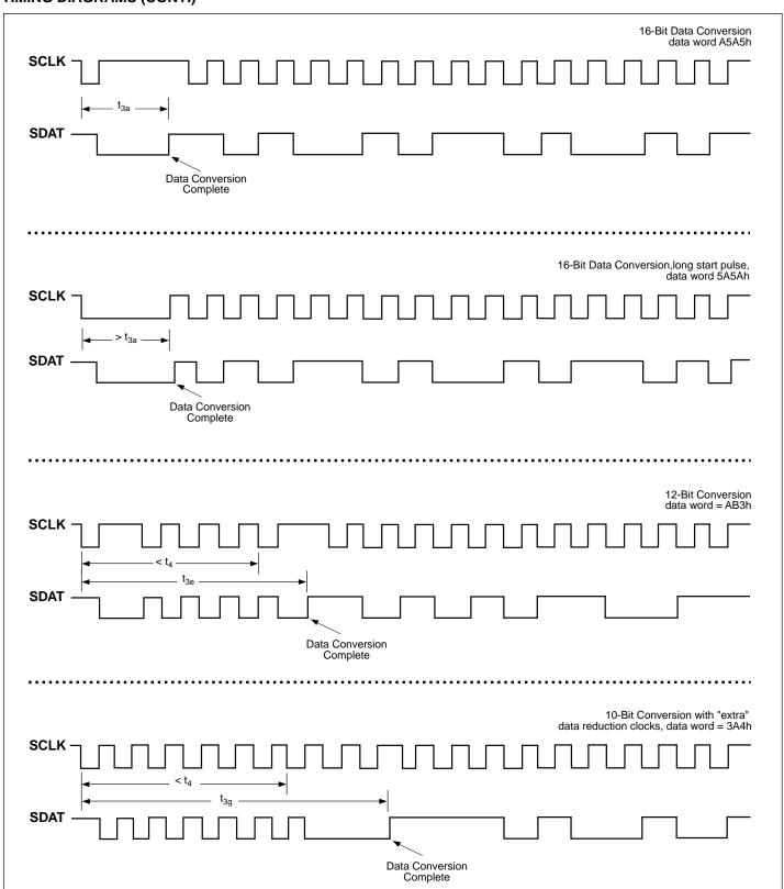
Figure 4. Example Timing Diagrams
