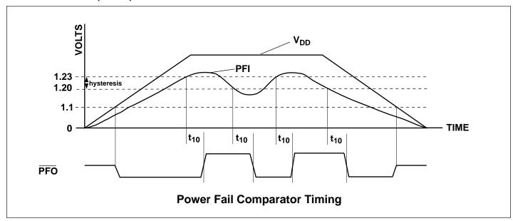
Figure 5. Power Fail Timing
