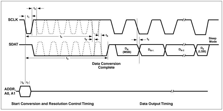
Figure 2. Conversion and Data Output Timing
