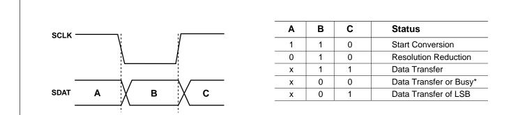
\*Note: The code x00 has a dual meaning: Data Transfer or Busy Converting. To avoid confusion, the user should send only the required number of pulses for the desired resolution, then wait for SDAT to rise to 1, indicating conversion complete before clocking SCLK again to read out data bits.
